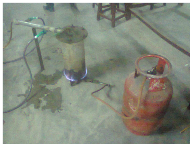
Figure.1.1 Experimental Set Up for the Plastic Hydrocarbon fuel.
